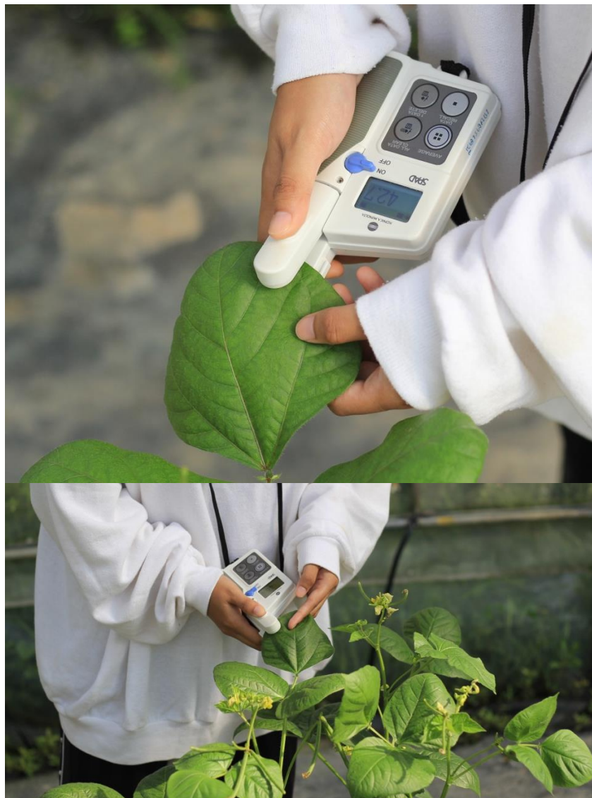
Fig 5 Measurement chlorophyll content by chlorophyll meter SPAD-502Plus (Konica Minolta) at V4 R1 R2 and R4stages
